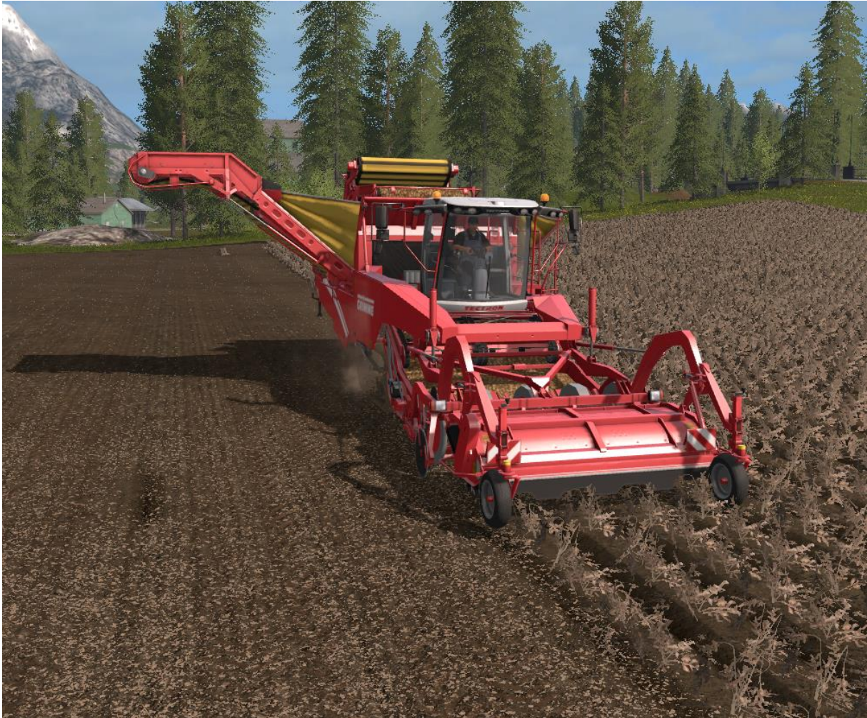
Figure 3: Haulm topping and harvesting in one machine (GIANTS Software, 2017).
